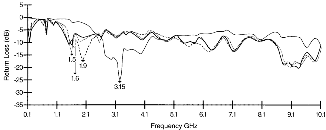
Fig. 10. Measured return loss in decibels of the assembled monopole at four different bias settings. The performance demonstrates frequency-hopping operation.
